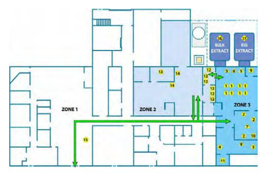
FIGURE 4: DIAGRAM OF TRITIUM AND PRODUCT MOVEMENT THROUGH FACILITY
